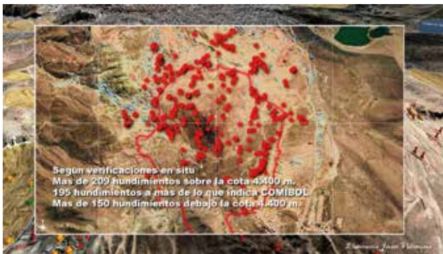
Fig. 5: According to on-site verifications, there are more than 209 collapse holes above 4,400m elevation, 195 more than indicated by COMIBOL, and more than 150 collapse holes below the level of 4,400m.
