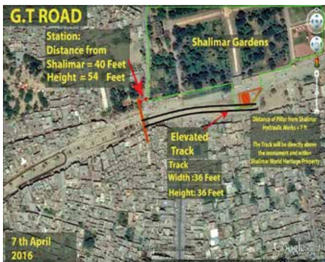
Fig. 1: The elevated track of the metro passing by the Shalamar Gardens and hydraulic works, April 2016.
