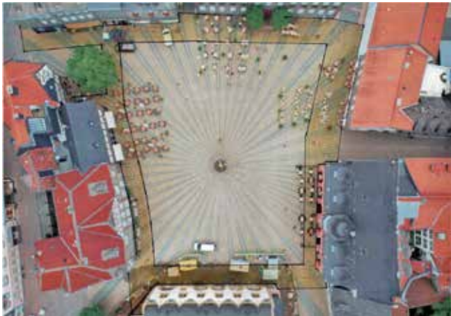
Fig. 4: Illustration of the intended change of the market square with the approx. 1,000 m 2 surrounding band of granite slabs. Computer animation: City of Goslar
