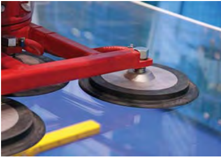
▲ Figure 5.42 Large suction pads can be used to move large pieces of glass.
