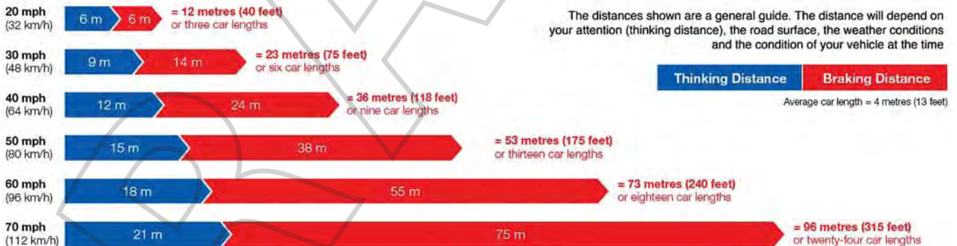
▲ Figure 5.84 These stopping distances appear in the Highway Code. You need to know these to drive safely. The reaction time here is about 0.7 s.
