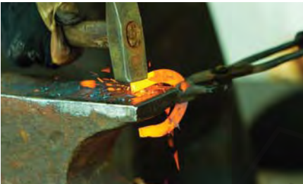
▲ Figure 6.70 This blacksmith can judge the temperature of the steel by looking at the colour of the radiation.
