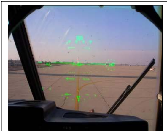
Wikimedia CC -2.0 Telstar Logistics photo C-130J Hercules Co-pilot's Head up display (HUD)
