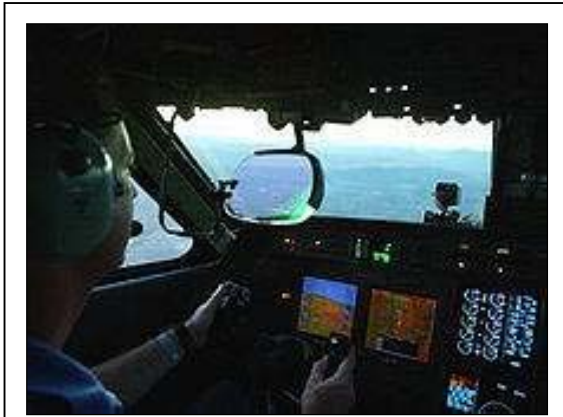
Wikimedia NASA PD photo NASA's Gulfstream G-V cockpit (with synthetic vision system display)
