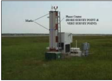
MLS Elevation guidance station with horizontal & vertical survey Phase Centre where shown) Fig 23.2 – D (USGS Photo)
