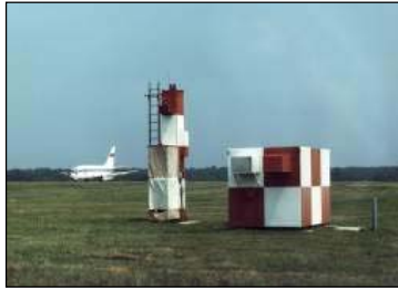
The NASA 737 research aircraft with the Microwave Landing System equipment in the foreground. Fig 23.2 –E (NASA photo)
