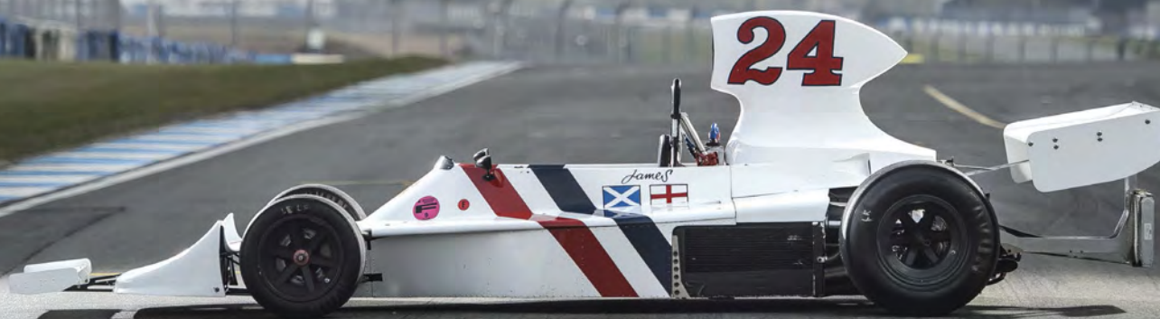
Harvey Postlethwaite's unusual high-rise airbox was a rare departure from an otherwise conventional layout
