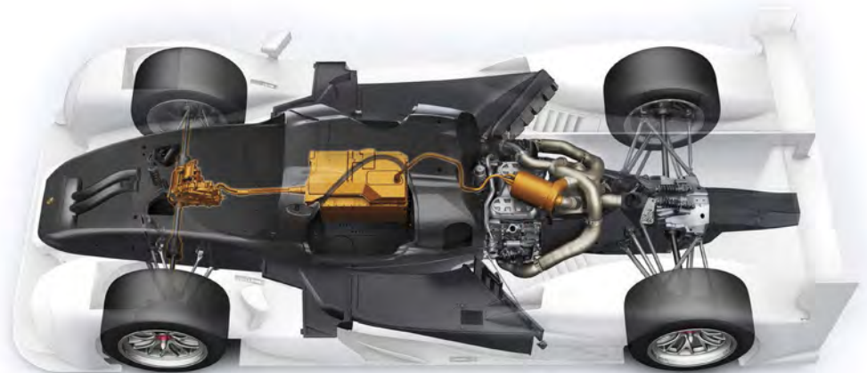
Porsche's hybrid system (right) employs water-cooled batteries recovering energy from both front axle and an exhaust turbine
