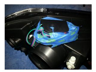
**Step 8:** screw in the 2 screws that go into the back of the headlight. Use your clear glazing silicon to fill up the gap between the headlight housing and the lens all the way around push it into the gap with your finger, seal up where the wires are coming out too then let it dry, rub off the excess silcone. Refit all your globes/hids.
