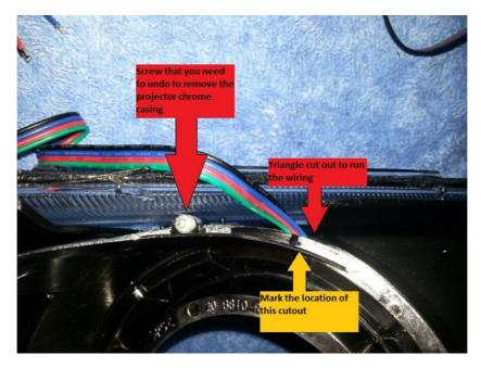
**Step 6:** The high beam section uses the "C shaped" angel eye the open end faces the top and sits behind the black casing and the curved bottom of it sits just on top but flush its the back of the black casing, This is the hardest one to glue into place, the best way is to tape it into place ensure its centered in the hole and a even amound of overlap either side sticking out the top. Glue in the top corners then the bottom center. Let it dry and remove the tape.
