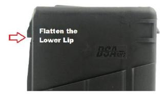
If your new polymer magazine is struggling to lock into your magazine catch on your metric FAL rifle try flattening out the lower lip of the rear catch. This should be simple enough to do with sandpaper, a small file or even a box cutter.
