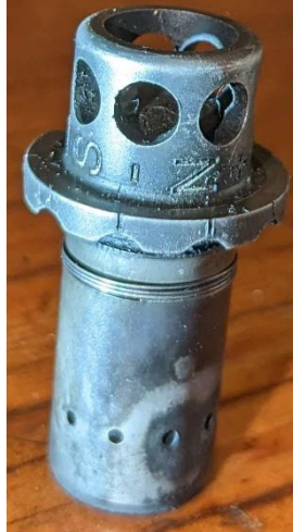
Figure 3: MDRx Gas Plug Crown/Castle Design
