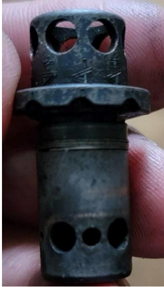
Figure 6: 300 BLK Gas Plug Design
