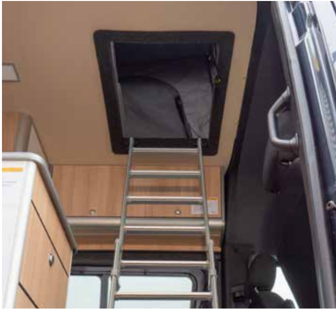
Access hatch with access ladder
