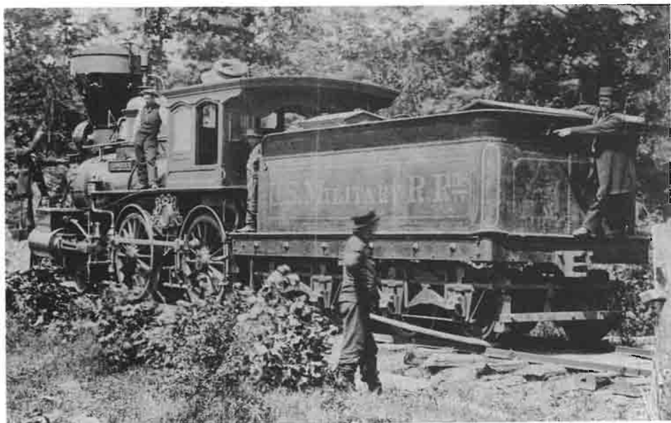
U.S. Military Rail Roads locomotive with crew members pointing at holes in the smokestack and tender caused by rebel shells
